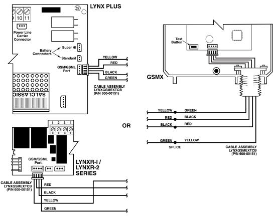
Figure 1. GSMX Connections
